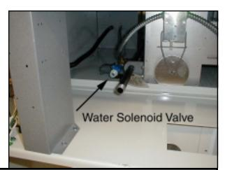
**NOTE:** The 3/4"-11.5 NH is a standard hose coupling screw thread. It <u>is not</u> to be confused with 3/4" N.P.T. The sealing of an NH connection is made with a washer opposed to the mating threads of an N.P.T. assembly. The two (2) thread designs <u>are not</u> compatible.
